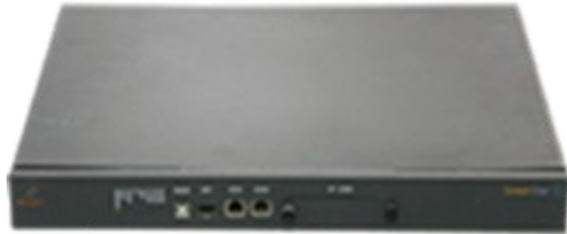
Base Station Baseband Unit (BBU)
